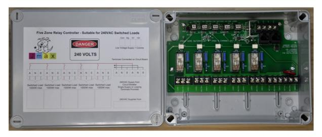
This unit will control 5 general purpose loads. It is suitable to switch 240VAC voltage via on/off control.
